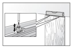
Tighten the nuts on the adjusting rail. This will correct the side alignment of the door.
